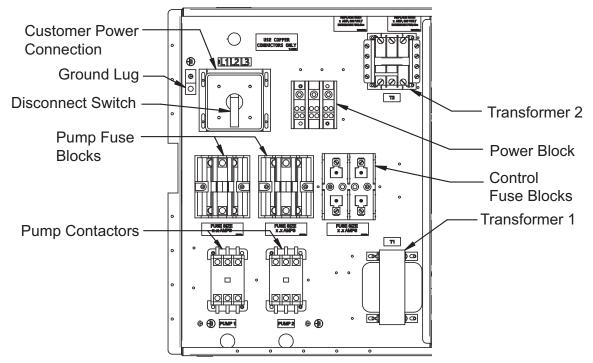
Figure 13 High voltage connections—50Hz
